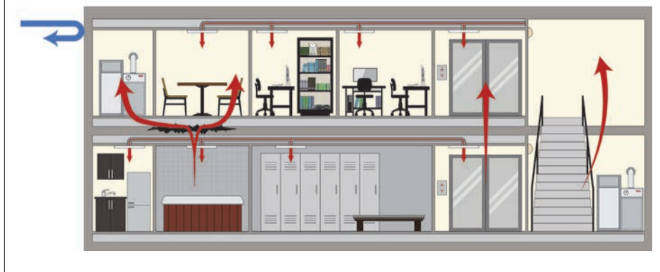
Observed Air Flow in Building of Outbreak Location
