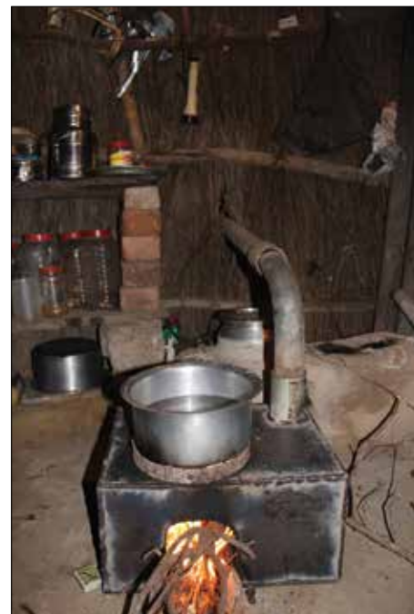
New improved metal cookstove prototype with smoke chamber and chimney to vent smoke out of the house.
