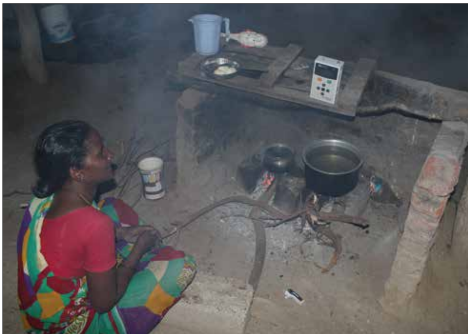
Woman cooking on an open cook fire with a monitor being used to measure pollution levels.
