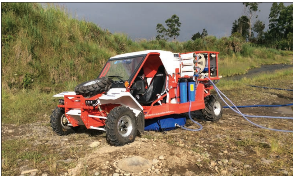
Portable desalination vehicle. Reprinted with permission from G.A.L. Water Technologies Ltd.
